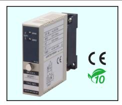
This compact plug-in, high-speed response type converter (isolator) provides signal output which is mutually isolated between input, output and power-supply. It amplifies and converts various kinds of signal with isolation to use in the integrated instrumental control system. It is highly effective as noise countermeasures.
