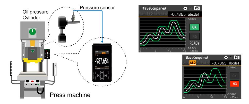
It is possible to judge not only the pressure level but also the concept of time. High-speed sampling of 4000 times / sec at the fastest
