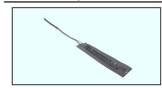
TKS is a sheet type thermocouple with a thickness of about 0.2 mm. It is insulated by ultrathin film, it is highly responsive and it is used for surface temperature measurement of various objects.
