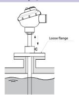
When changing the depth of the measurement position on a trial basis or adjusting the depth on site, use it in combination with the optional loose flange. However, loose flanges and loose screws are not airtight.
