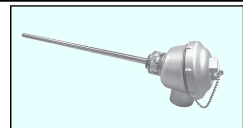
R01 is a resistance temperature detector with the simplest shape for a terminal box. By combining with loose flange (LFL) and compression fitting (CFG), it can be used for temperature measurement of ducts and tanks as an insertion type with adjustable insertion length.
