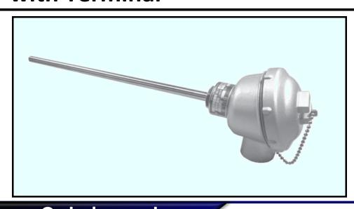
R01 is a resistance temperature detector with the simplest shape for a terminal box. By combining with loose flange (LFL) and compression fitting (CFG), it can be used for temperature measurement of ducts and tanks as an insertion type with adjustable insertion length.
