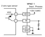
\* Use [V HI] terminal as HI terminal if the sensor is voltage output type, use [A HI] terminal if the sensor is current output type.
