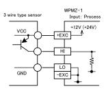
\* Use [V HI] terminal as HI terminal if the sensor is voltage output type, use [A HI] terminal if the sensor is current output type.
