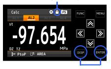
KEY LOCK off: Disabled by pushing DISP key and ENTER key simultaneously
