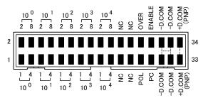
Suitable wire: AWG#28 flat cable(7/0.127mm)
