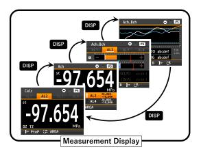
\*Example: Measurement display (calculation), measurement display (Ach + comparison), level display (Ach + Bch), trend display (Ach + Bch)
