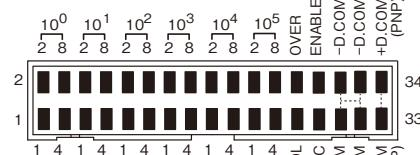
Compatible wire: AWG28 flat cable (1.27mm)
