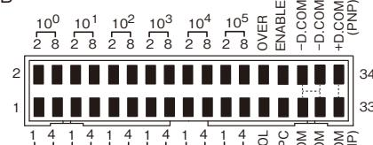
Compatible wire: AWG28 flat cable (1.27mm)
