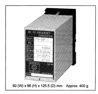
This converter takes in an analog current or voltage, and outputs a pulse having a frequency that is proportional to its input value. This converter is highly suitable for adding up analog flow rate signals or electrical energy. Its output signal form is compatible with electronic or electromagnetic counters. The converter has its input and output isolated by a photocoupler.
