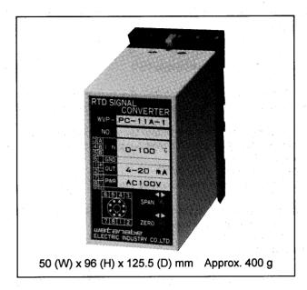
This plug-in temperature signal converter is employed in combination with a platinum resistance temperature sensor. It is a high-performance converter that comes standard with a linearizer and a burnout circuit, and adopts circuitry that is hardly affected by conductor resistance. In addition, this unit can be equipped with a built-in photocoupler-type isolator.
