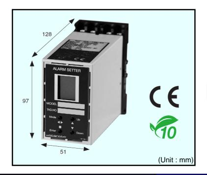
This converter inputs DC signal and outputs a relay contact signal or open-collector signal if the DC signal input value exceeds the preset value (one point). Parameter change and input values can be monitored on the front LCD panel.
