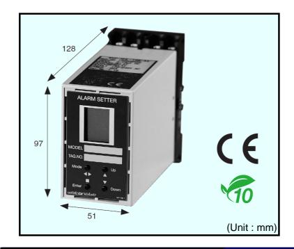
This converter inputs DC signal and outputs 2 points relay contact signals or open-collector signals if the DC signal input value exceeds the preset value (one point). Parameter change and input values can be monitored on the front LCD panel.
