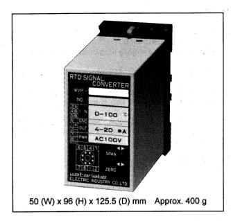
This plug-in temperature signal converter is employed in combination with a nickel resistance temperature sensor. It is a high-performance converter that comes standard with a linearizer and a burnout circuit, and adopts circuitry that is hardly affected by conductor resistance. In addition, this unit can be equipped with a built-in photocoupler-type isolator.
