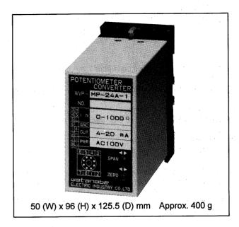
This unit precisely converts the amount of rotational motion or linear movement that is taken in the form of resistance variation from a potenliometer into a current signal or voltage signal. It is a high-performance plug-in converter that allows users to choose from many outputs the optimum one for centralized monitoring equipment, computers, data loggers, and measurement control devices. The MZ and MS models have their inputs and outputs isolated by the photocoupler method.
