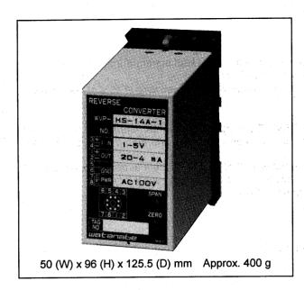
This converter comes in handy when input and output signals need to be placed in a mutually inverse relationship. For example, as the input signal increases from 4 mA to 20 mA, the unit can work to conversely reduce the output signal from 20 mA to 4 mA. Its input and output can be isolated using photocoupler method.
