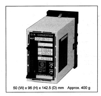
This unit converts parallel BCD signals or binary-code signals from a sequencer and computer, or gray-code signals from a rotary encoder, into analog DC signals. High-speed conversion and high resolution have been achieved through the use of a built-in microprocessor unit.
