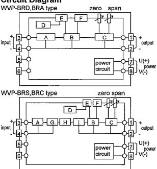
A: input circuit, B: ratio bias circuit, C: output circuit
