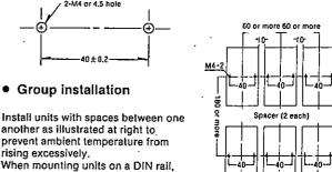
Install units with spaces between one another as illustrated at right to prevent ambient temperature from rising excessively.
