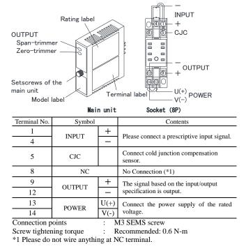
6-16-19, JINGUMAE, SIBUYA-KU, TOKYO 150-0001, JAPAN TEL: +81-3-3400-6147 FAX: +81-3-3409-3156 \*This equipment has burnout protection circuit built-in, which upscale output signal higher than the 100% when connected thermocouple has been disconnected.
