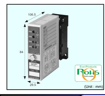
This compact plug-in signal converter accepts AC tachogenerators intput and converts into optically isolated two DC signal outputs. And also provides isolation between the signal input, output, and power supply.
