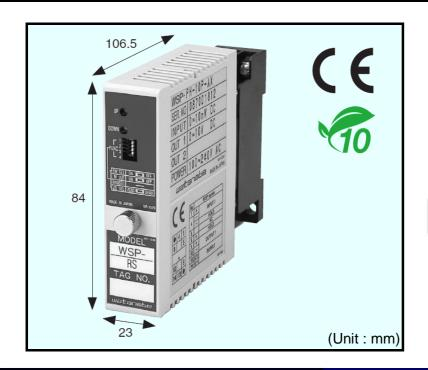
This compact plug-in signal converter accepts signal with square-law characteristics and provides optically isolated signal output, corresponding to the square root. It amplifies and converts the selected DC input to the selected DC output. It can use for extraction of square root of differential pressure type / open-channel flowmeter (linearization).
