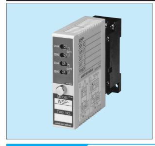
This compact plug-in signal converter with two insulated outputs converts the secondary outputs of PTs (VTs) in power substations, motor circuits, etc. into instrumentation signals. Since Type PTEW adopts the true root-meansquare value operation system, it ensures particularly high reliability against distorted waves.
