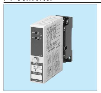
This compact plug-in signal converter converts the secondary outputs of PTs (VTs) in power substations, motor circuits, etc. into instrumentation signals. Since Type PTE adopts the true root-mean-square value operation system, it ensures particularly high reliability against distorted waves.
