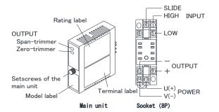
Terminal No. Symbol Contents HIGH Please connect a HIGH(100%) connection. 1 4 INPUT SLIDE Please connect a SLIDE connection. 5 LOW Please connect a LOW(0%) connection 8 NC No Connection (\*1) 9 + The signal based on the input/output OUTPUT 12 specification is output. U(+) 13 Connect the power supply of the rated POWER 14 V(-) voltage. Connection points M3 SEMS screw
