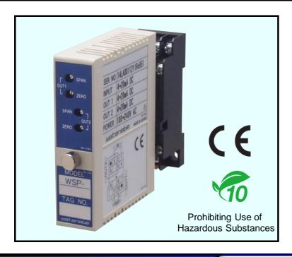
This compact plug-in, high-speed response type converter (isolator) provides 2 signal outputs which are mutually isolated between input, output and power-supply. It amplifies and converts various kinds of signal with isolation to use in the integrated instrumental control system. It is highly effective as noise countermeasures.
