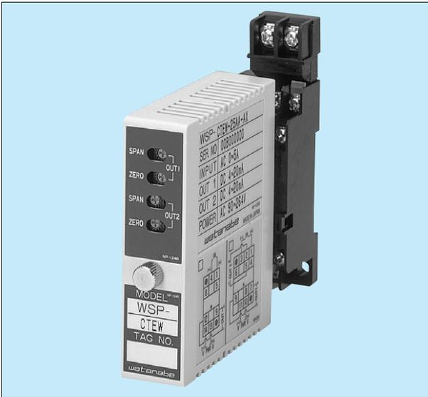
This compact plug-in signal converter with two insulated plug-in outputs converts the secondary outputs of CTs in power substations, motor circuits, etc. into DC signals. Since Type CTEW adopts the true root-mean-square value operation system, it ensures particularly high reliability against distorted waves.
