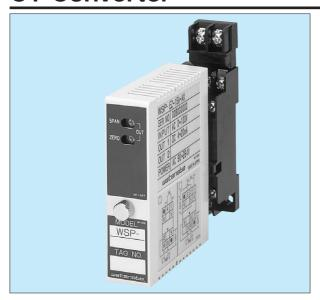
This compact plug-in signal converter converts the secondary outputs of CTs in power substations, motor circuits, etc. into instrumentation signals. Since Type CTE adopts the true root-mean-square value operation system, it ensures particularly high reliability against distorted waves.
