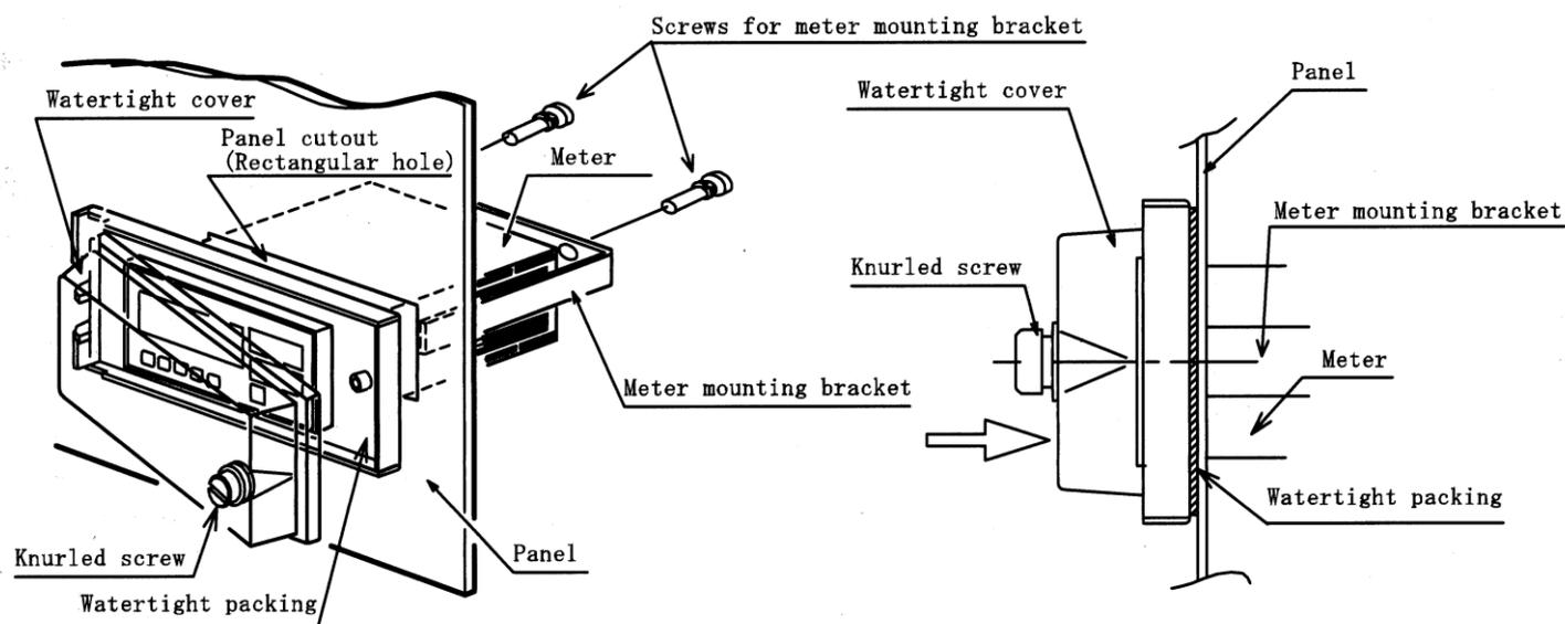
Note: After the watertight cover is mounted, check that there is no gap between the cover and panel.
