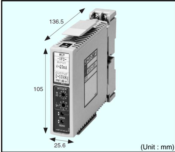
This slim-type plug-in converter accepts DC voltage or current input and provides isolated two pulse outputs. It amplifies and converts the selected DC input to the selected pulse outputs. And also provides isolation between the signal input, output, and power supply.
