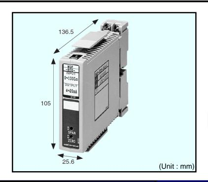
This slim-type plug-in signal converter converts a signal detected as a change in the resistance value to a DC voltage or current signal. Measurement of float-type level sensor arm position / Alarm system for sharp change in resistance value / Enables measurement of low resistance and high resistance.
