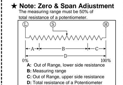
A procedure for adjustment, adjust Zero first,
