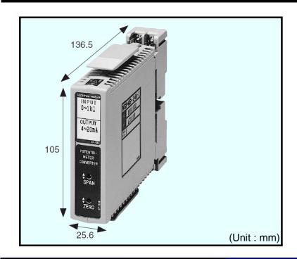
This compact plug-in signal converter converts the amount of rotation movement or linear travel distance extracted as a change in the potentiometer's resistance value to the selected DC voltage or current output. And also provides isolation between the signal input, output, and power supply.
