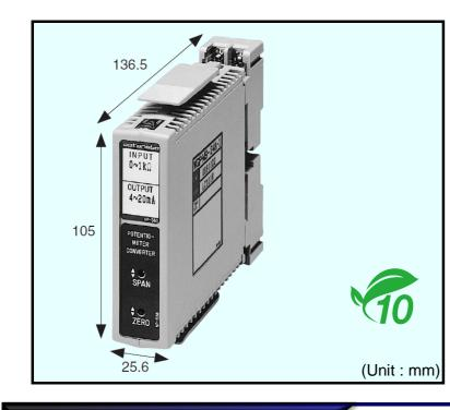
This compact plug-in signal converter converts the amount of rotation movement or linear travel distance extracted as a change in the potentiometer's resistance value to the selected DC voltage or current output.
