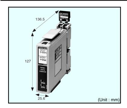
This compact plug-in converter accepts Thermocouples input conforming to JIS standard and provides optically isolated DC voltage or current output. This converter has a linearizer, a cold junction compensating circuit, and a burnout protection circuit as standard equipment which is required to measure temperature.
