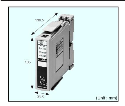
This slim-type plug-in signal converter converts AC voltage or current to a DC signal best suitable for the measurement control equipment input. With the true RMS value operation method, this converter ensures high reliability against distorted waves.
