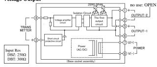
· Current Output no use: SHORT OUTPUT-2 TRANS MITTER OUTPUT-1 PÓWER Input Res V(-)V DBZ: 250O DBT: 300Ω
