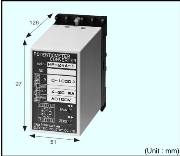
This plug-in signal converter converts the amount of rotation movement or linear travel distance extracted as a change in the potentiometer's resistance value to the selected DC voltage or current output. Model MZ and MS type is isolated between input and output by photocoupler.
