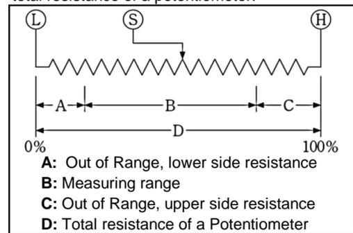
A procedure for adjustment, adjust Zero first, and then adjust the Span.
