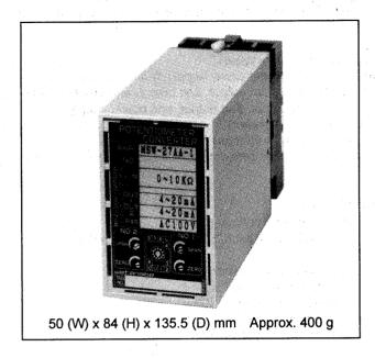
This plug-in type signal converter with 2 isolated outputs converts the amount of rotational motion or linear movement that is taken out in the form of a resistance variation from a potentiometer into a current signal or voltage signal. Since you can choose an optimum output from this converter, which has its input, output and power supply isolated from one another, for feeding it to a measurement control device, the unit can be employed in a wide variety of applications.
