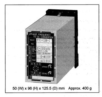
This unit is a small-sized plug-in signal converter that converts a two-phase pulse signal mutually dephased by 90 degrees, emitted from an incremental type rotary encoder, into an analog signal that allows to identify the rotating direction by a magnitude proportional to its frequency.
