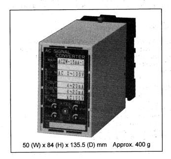
These units are plug-in type signal converters with 2 isolated outputs that convert AC voltage signals or current signals into DC signals that can be handled in a standardized manner in a system, and besides, that are fit to a long-distance transmission. Since Type EFZW adopts the true root-mean square operation system, it assures particularly high reliability against distorted waves.
