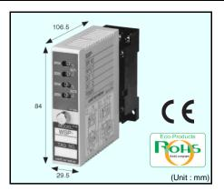
This compact plug-in signal converter (distributor) with two outputs supplies 24Vdc to the 2-wire transmitter through signal lines and converts the signals (4 to 20 mAdc) to the DC voltage or current output.
