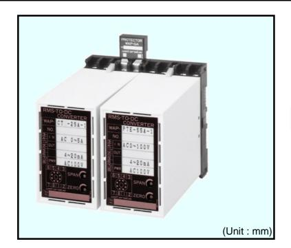
This plug-in converter (isolator) accepts AC voltage or current input and provides optically isolated DC voltage or current output.
