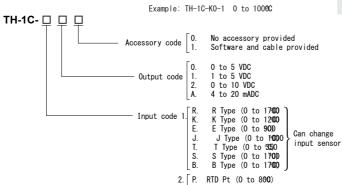
As input specifications, separately specify the zero and span temperatures (in steps of  ${\tt CD}$ ).
