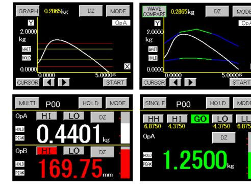
High-speed processing of 4,000 times/sec (When one chis used) Possible to connect in parallel up to four load cells with a resistance of
