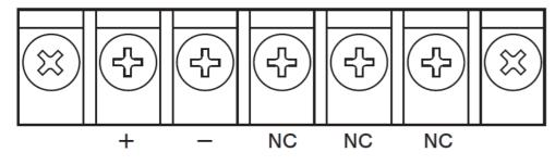
Notes: Unable to use NC terminal as intermediate terminal. In case analog output model, either 4-20mA or 0-10V is available.
