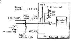
Each input terminal (BCD  $10^{\rm 0}$  to  $10^{\rm 4}\,\rm digit,$  latch and polarity) is internally pulled-up.
