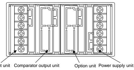
Each unit is not replaceable by the customer.
