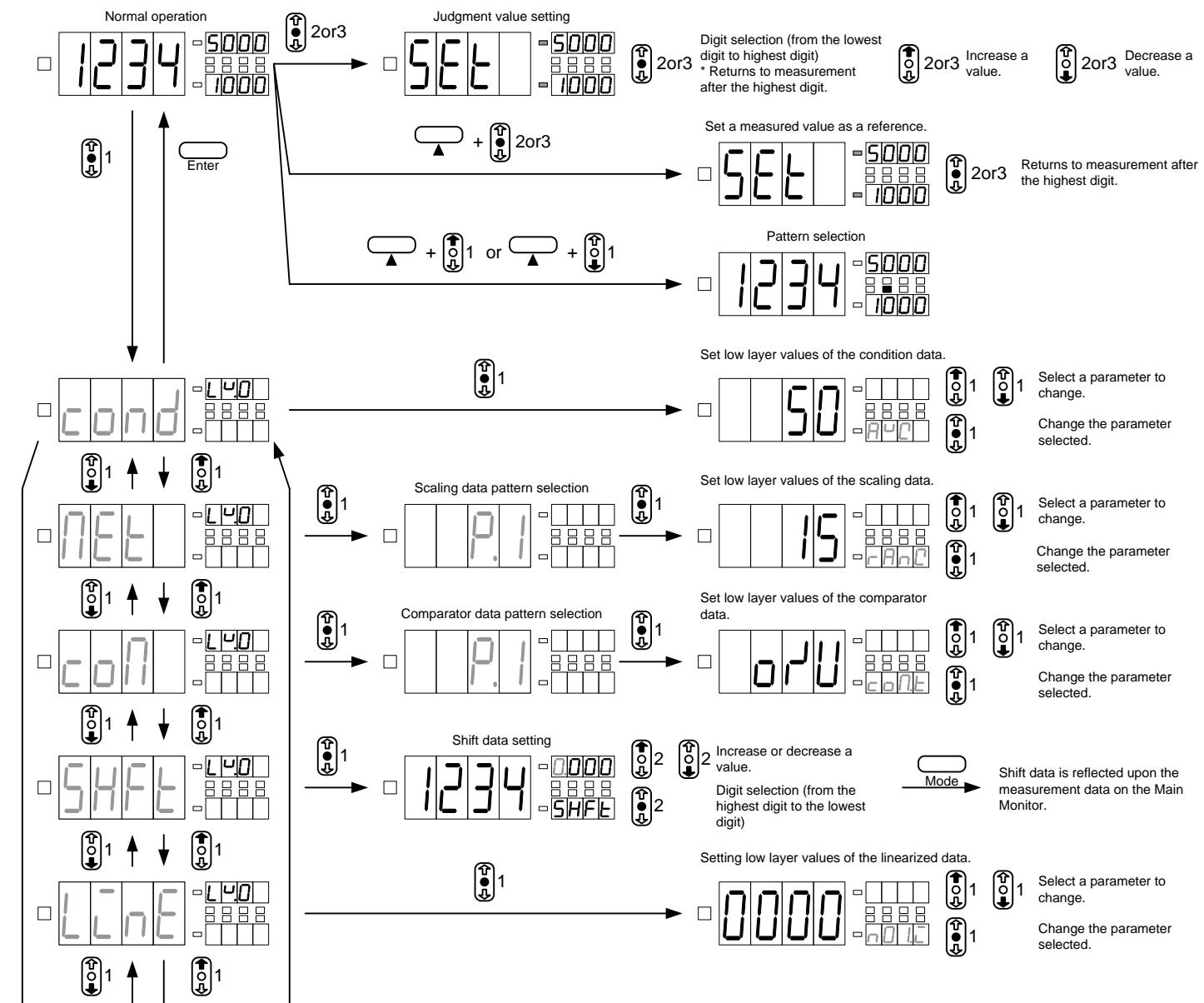
How to set a low layer value (Condition data/scaling data/comparator data)
