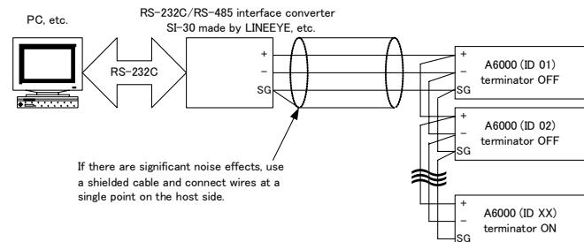
If there are significant noise effects, use a shielded cable and connect wires at a single point on the host side.
