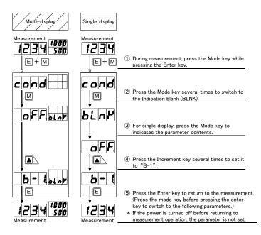
\* When the indication blank function is ON, the main display and sub display (Multi-display only) will be completely turned off. To turn them on, follow the steps above from step  $\widehat{\mathbb{T}}$ . (During parameter setup, the display blank function is turned off and the indication is turn on.) OFF(bright)  $\rightarrow$  B-3  $\rightarrow$  B-2  $\rightarrow$  B-1 (dark)  $\rightarrow$  ON (turn off)
