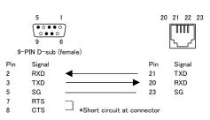
\* The host side CTS and RTS terminals connection is a typical example of a connection for hardware control. Please check with the system designer for details before making the connection
