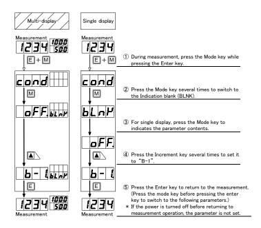
\* When the indication blank function is ON, the main display and sub display (Multi-display only) will be completely turned off. To turn them on, follow the steps above from step  $\mathbb{O}$ . (During parameter setup, the display blank function is turned off and the indication is turned off and the indication is turned off.) OFF(bright)  $\rightarrow B-3 \rightarrow B-2 \rightarrow B-1$  (dark)  $\rightarrow ON$  (turn off)
