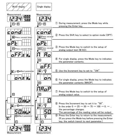
\* When you exit the output value (%) indication, the analog output test will turn off and return to the original output value.
