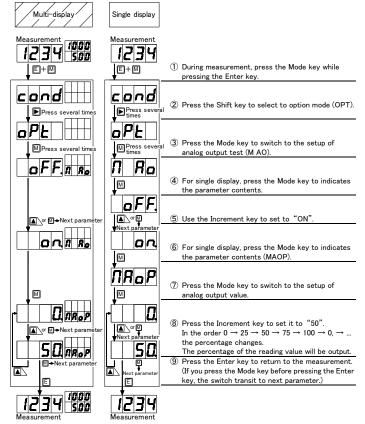
\* When you exit the output value (%) indication, the analog output test will turn off and return to the original output value.
