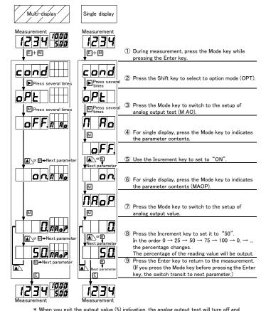
\* When you exit the output value (%) indication, the analog output test will turn off an return to the original output value.
