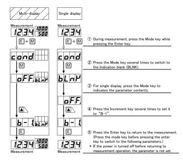
\* When the indication blank function is ON, the main display and sub display (Multi-display only) will be completely turned off. To turn them on, follow the steps above from step  $\widehat{\mathbb{T}}$ . (During parameter setup, the display blank function is turned off and the indication is turn on.) OFF(bright)  $\rightarrow$  B-3  $\rightarrow$  B-2  $\rightarrow$  B-1 (dark)  $\rightarrow$  ON (turn off)
