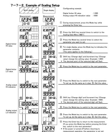
. Digital limiter HI value setup MODEL A5 - - 13 - - -6/12
